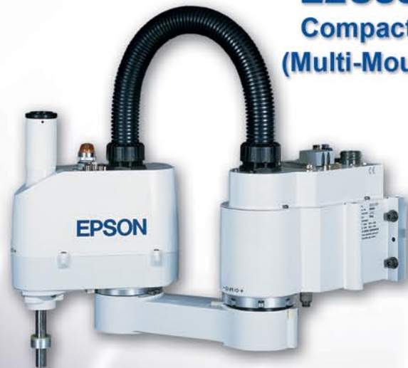
E2C351C Cleanroom Robot (Table Top Type)
